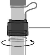
Before pulling out or putting back the electrode, make sure to fully loosen the blue cap on the storage sleeve so that the electrode can move in and out smoothly.
