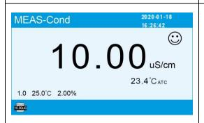
Calibration completed, instrument goes back to measurement mode.
