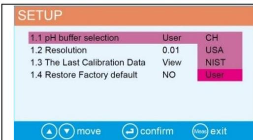
1. Select User in parameter setting 1.1, press **CAL MEAS** key to return to measurement mode.
