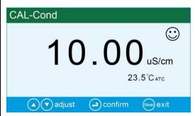
3. Submerge probe in 10μS/cm standard solution. Stir the solution briefly and allow it to stay in the buffer solution until appears and stays. Press or γ/κμ key to adjust measuring value to10.00μS/cm. Press key to finish calibration.
