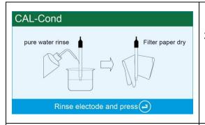
2. Long press Key to enter calibration mode, as shown in left graph. Rinse probe in purified water, remove excess water by shaking or filter paper. Press key to confirm.
