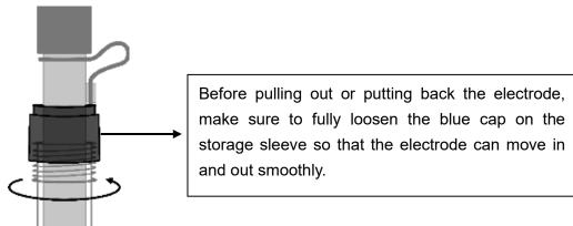
2.2 After long time exposure in air, Polymer electrolyte will cause shrinkage. It will not happen in measurement status. The electrode must be soaked in 3M KCl solution for storage. After long time soaking, there will be some floccules dissolving out from 3M KCl solution, this is normal phenomenon.
