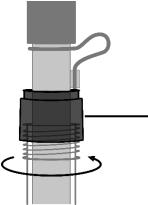
Before pulling out or putting back the electrode, make sure to fully loosen the blue cap on the storage sleeve so that the electrode can move in and out smoothly.
