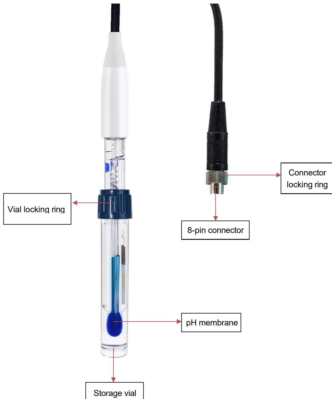
Crafted with proprietary sensor technology and premium materials from Switzerland, Apera LabSen 855 Glass pH/temp. Electrode is designed for high-precision pH measurement of viscous liquid such as cosmetics, skin care products, paints, coatings, glues, slurry, honey, liquid resin, etc.
